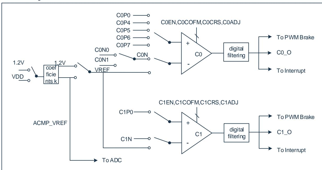
comparator with hysteresis control diagram is shown below:
