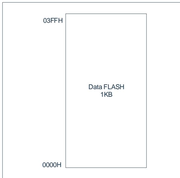
Data FLASH memory read, write, and erase operations are realized through the FLASH control interface.
