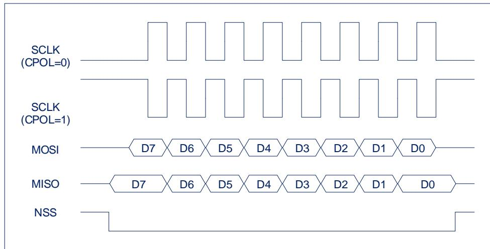
When CPHA=0, the NSS line must be de-set and reset between each successive serial byte. In addition, if the slave writes data to the SPI data register (SPDR) when NSS is at low level, a write conflict error will occur. When CPHA = 1, the NSS line may remain low between consecutive transmissions (it can always remain low). In a system with a single fixed master and a single slave driving the MISO data line, this format is sometimes preferred.
