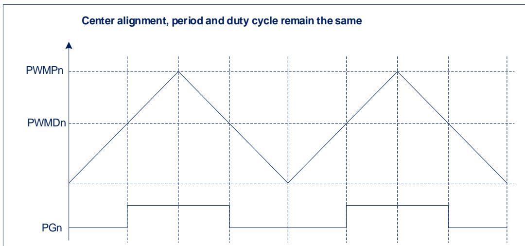
Center alignment symmetrical counting, the timing diagram of duty cycle change is shown in the figure below:
