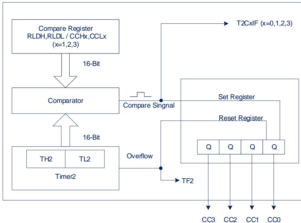
the output structure block diagram of comparison mode 0 is shown in the following figure:
