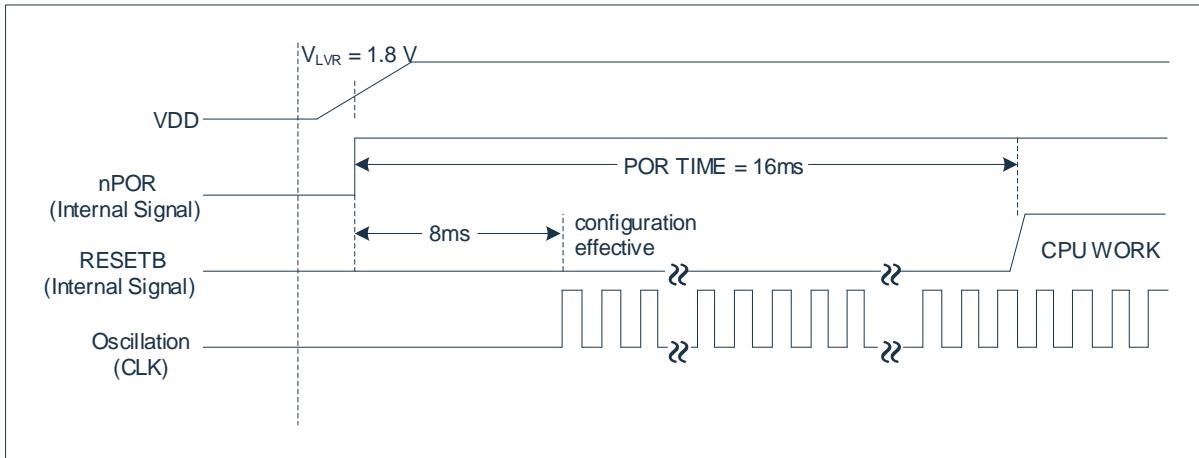
Whether the system is power-on reset can be judged by PORF (WDCON.6) flag bit. The reset types that can set the PORF flag to 1 are: power-on reset, LVR reset, power-on configuration monitoring, external reset, CONFIG protection reset, Window WDT reset.
