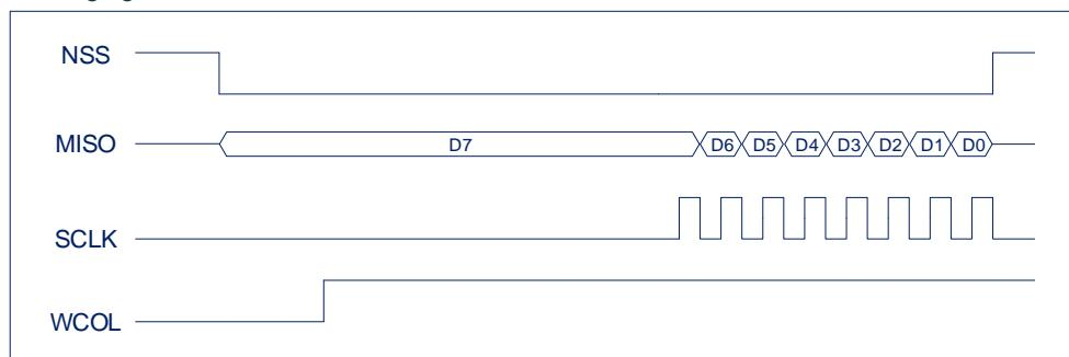
In addition, after writing SPDR in the slave mode, the NSS controlled by the master does not immediately become low. When NSS is low, you need to wait for the second edge of SCLK to start before entering the real data transmission state.
