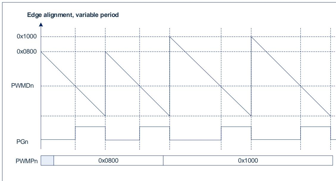
Edge alignment, duty cycle change timing diagram is shown in the figure below:
