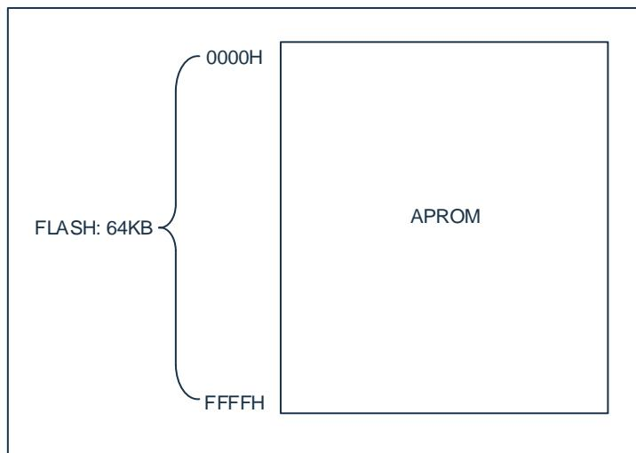
After the chip is reset, the CPU starts to execute from 0000H. Each interrupt is assigned a fixed address in the program memory, and the interrupt causes the CPU to jump to this address and start executing the service program.
