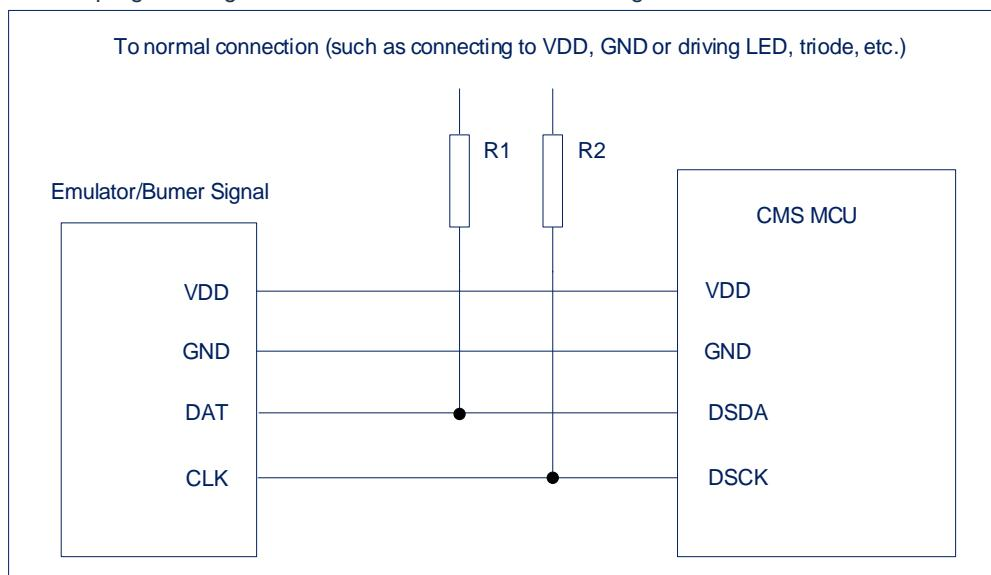
In the above figure, R1 and R2 are electrical isolation devices, which are often replaced by resistors. The resistance values are as follows:  $R1 \geq 4.7K$ ,  $R2 \geq 4.7K$ .
