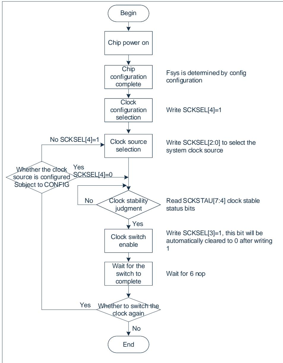
Note: When the system clock source is switched, it must be ensured that the corresponding clock source exists and has been correctly configured.
