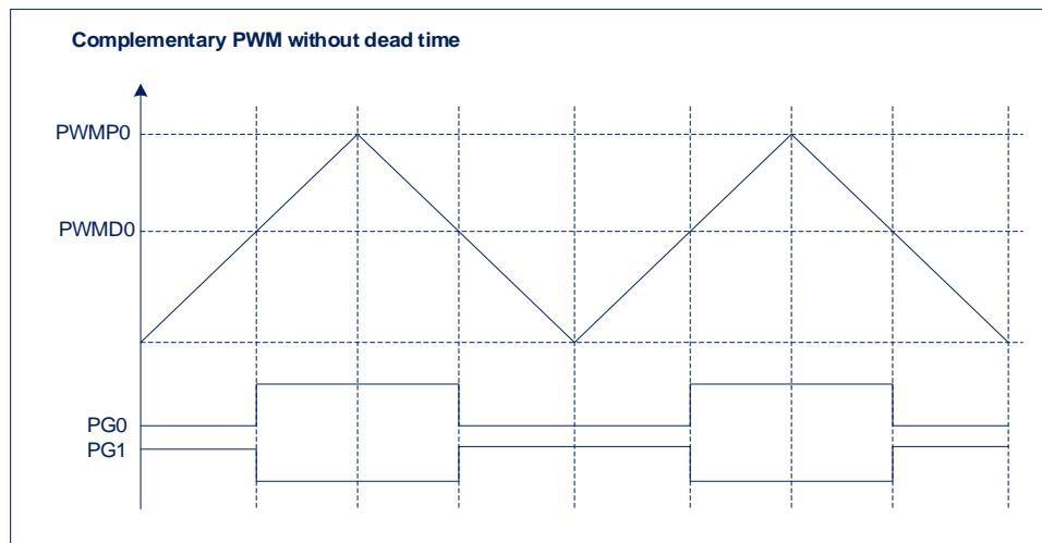
In motor control applications, the ideal PWM signal is the level flip at the same time. Due to the delay in the turn-on and turn-off of the MOS tube, it is easy to cause the power supply to be connected to the ground, thereby damaging the power tube. In order to avoid this phenomenon, PWM with dead time is particularly important. In complementary mode, each complementary PWM pair supports insertion of dead time, and the inserted dead time is as follows :
